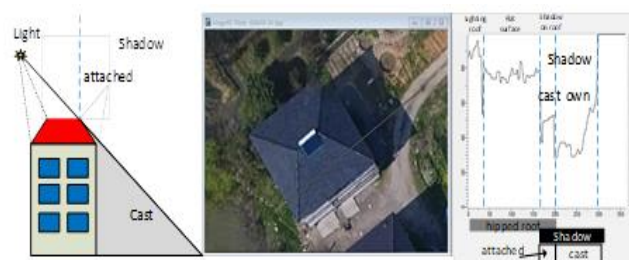
Fig. 2. Representation of the building with hipped roofs
