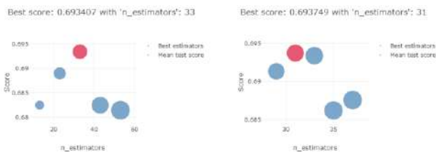
Fig. 11. Grid search process of 'n_estimators' hyperparameter for AB
