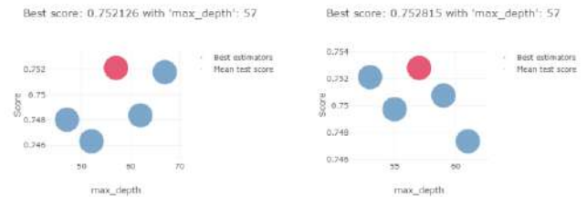
Fig. 6. Grid search process of 'max_depth' hyperparameter for RF
