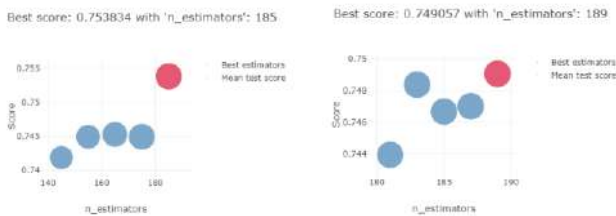
Fig. 8. Grid search process of 'n_estimators' hyperparameter for ET
