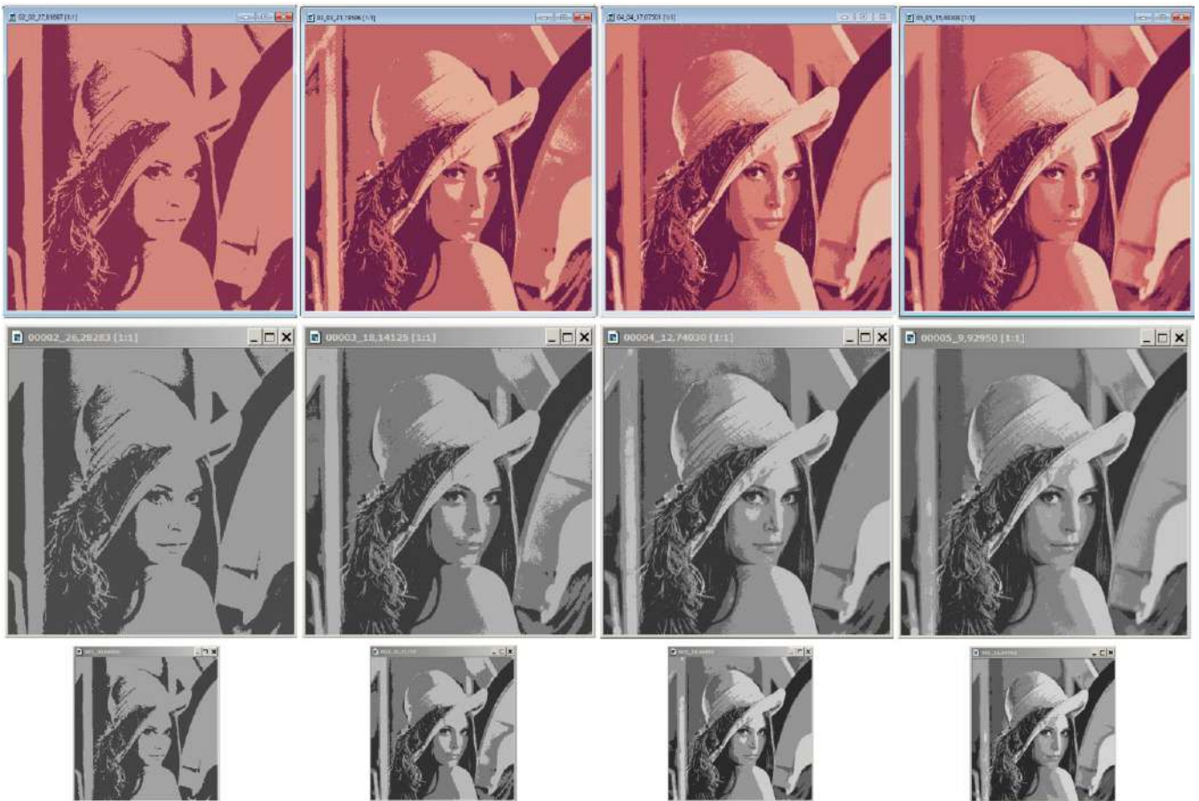
Fig. 4. Stability of segmentation through optimal clustering when converting a color image to a grayscale representation (top pair of approximation rows) and invariance to scaling (bottom pair of approximation rows).
